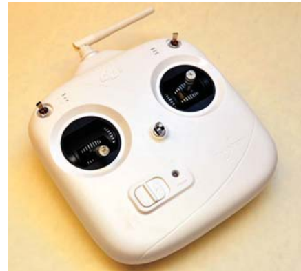
The transmitter is powered by four standard "AA" batteries.
